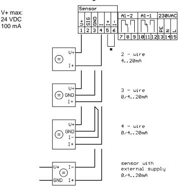
\* A bridge circuit is inserted ex factory . For signal transfer please remove the bridge circuit and attach the connection cables. Attention: Current loop has to be closed!
