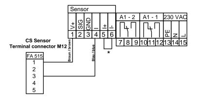
\* A bridge circuit is inserted ex factory . For signal transfer please remove the bridge circuit and attach the connection cables. Attention: Current loop has to be closed!
