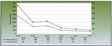
By means of the History Report the continuous improvements which have been reached during several months/years due to consequent leakage detection and leakage elimination can be documented.
