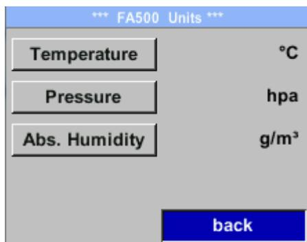
To make changes to the unit for the respective measurement value, first select by pressing „ $\Delta$ “ the field of the „measurement value“ and activate „it with „OK”.
