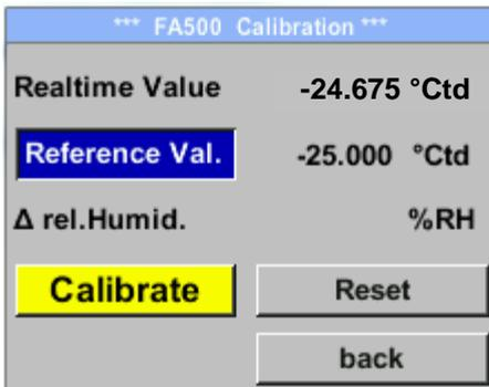
Here, a one-point calibration can be performed
