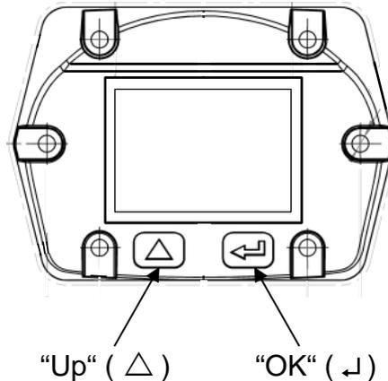
The operation of the FA 500 is done by the two capacitive key buttons Up (△) and Enter (↵)
