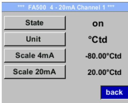
The 4-20 mA Analogue output of the Sensor FA 500 can be individually adjusted.
