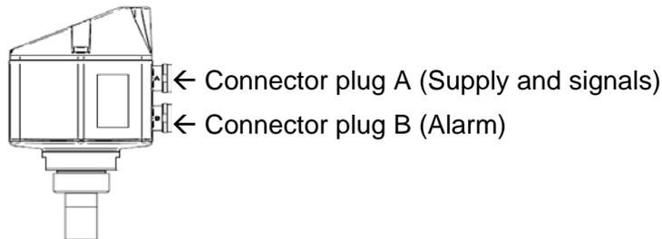
**Attention:** Not required connections NC must not be connected to a voltage and/or to protection earth. Cut and insulate cables.
