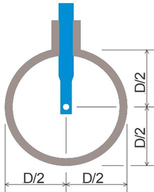
The sensor is then inserted to the required immersion depth and aligned according to the direction of air flow as described on page 3. A depth scale engraved on the probe tube, a flow alignment arrow and an aligning device will be of help to you.
