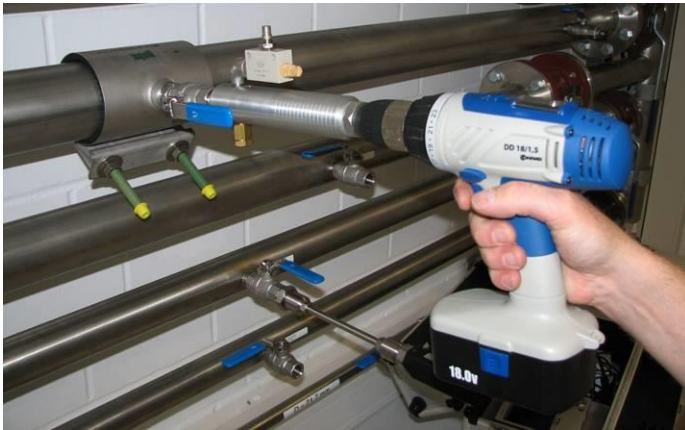
Drilling with CS drilling jig Order no. 0530 1108
