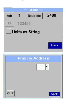
Select the desired position by pressing the button  $\_\Delta$  "and select it with "OK" button.
