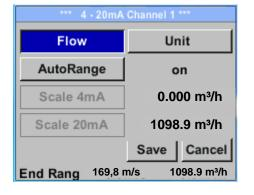
The 4-20 mA Analogue output of the Sensor VA 570 can be individually adjusted.
