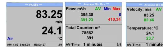
AV-Time ( Period for average value calculation) could be changed under Sensor Setup.-Advanced— AV-Time
