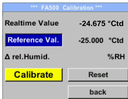
Here, a one-point calibration can be performed
