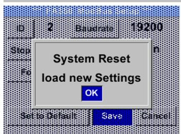
For changes, e.g. the sensor ID, first select by pressing key „ $\Delta$ “ the field “**ID**” and then key “**OK**”.
