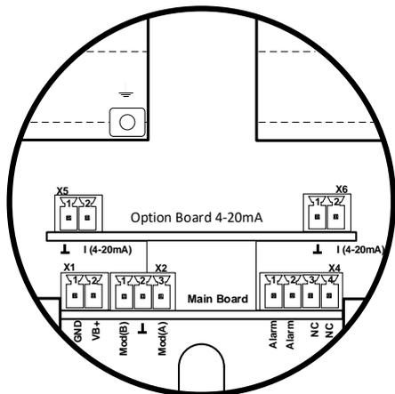
Version with option board 2x analogue outputs galvanically isolated
