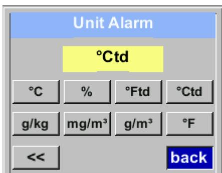
To select a measurement value, a corresponding / appropriate unit needs to be defined. Select „**Unit**“ with „**Δ**“ and open the menu with „**OK**“. Select required unit with „**Δ**“ and takeover it by pressing „**OK**“.
