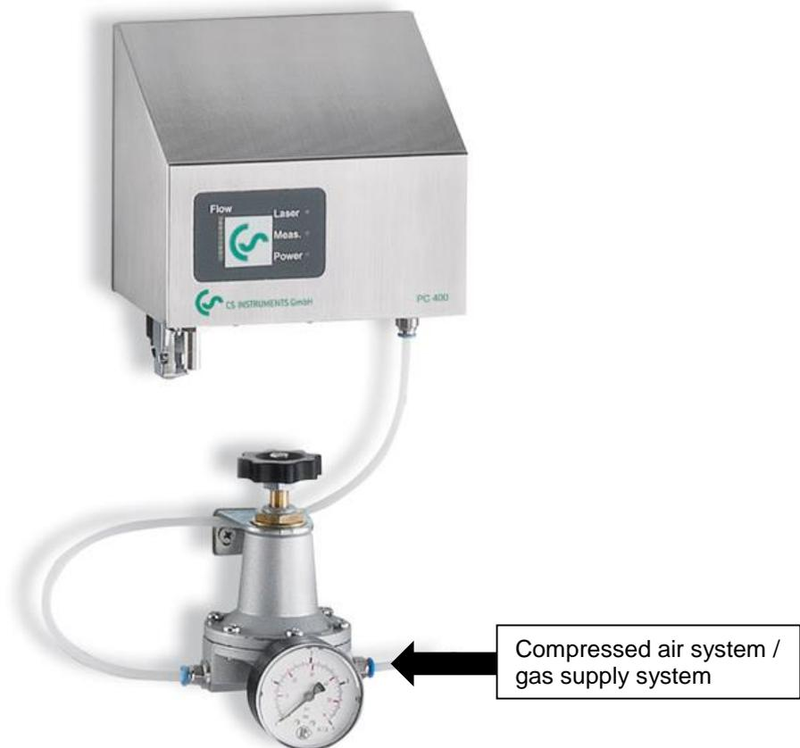
**Important:** The pressure at the particle counter PC 400 is not allowed to exceed 1.6 bar over-pressure. The pressure has to be reduced correspondingly by means of the supplied pressure controller.
