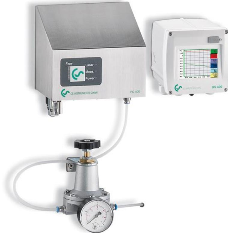
The data transfer of the measured values between PC 400 particle counter and DS 400 is effected via a digital RS 485 interface (Modbus protocol).
