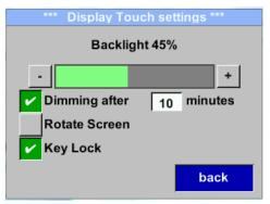
With the button "-" and with button "+" it is possible to adjust the backlight / display brightness. The actual / adjusted backlight brightness is showed in the graph "Backlight."
