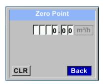
When, without flow, the installed sensor shows already a flow value of > 0 m³/h herewith the zero point of the characteristic could be reset.
