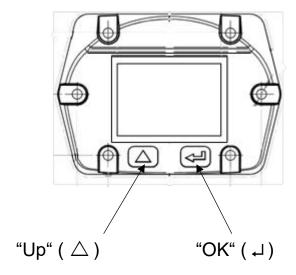
The operation of the VA 521 is done by the two capacitive key buttons Up  $(\triangle)$  and Enter  $(\della]$
