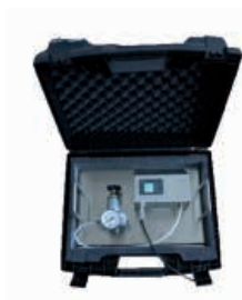
Compressed air quality measurement
