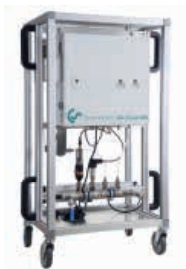
Compressed air quality measurement
