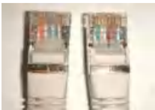
Crossover cable with RJ45-plug
