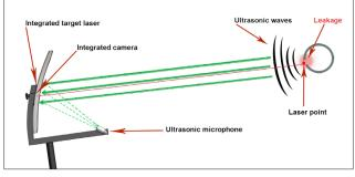
By focusing the ultrasonic waves in the parabolic mirror, even the smallest leaks of 0.8 l/min (approx.  $\in$  8 p.a.) can be located with pinpoint precision (± 15 cm) at a distance of up to 10 to 15 m.
