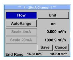
The 4-20 mA Analogue output of the Sensor VD 500 can be individually adjusted.
