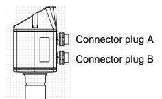
Attention: Not required connections NC must not be connected to a voltage and/or to protection earth. Cut and insulate cables.
