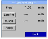
With the low-flow cut off activated, the flow below the defined "LowFlow Cut off" value will be displayed as 0 m<sup>3</sup>/h and not added to the consumption counter. For an input / change of the value select with the button  $_{n}\Delta^{"}$  the respective number position and activate it with  $_{n}OK"$ .
