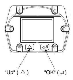
The operation of the VD 500 is done by the two capacitive key buttons Up (riangle) und Enter (riangle)
