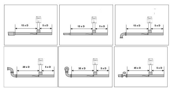
The values represent the min. lengths. In case the min. inlet / outlet runs could not be ensured, it must be expected to get increased or significant deviations of the measurement values.
