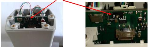
Alternatively, a 120R resistor can be installed in the plug between pin 2 and pin 4. It must be ensured that the connection plugs are still plugged and the gasket is installed correctly, see also chapter 4.5.
