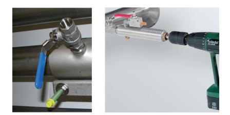
In case the system could not be shut down, means to be set depressurized, there could be used the CS spot drilling collar (Order-No. 0530 1108) and drilling jig (Order-No. 0530 1108) to drill through the ball valve.
