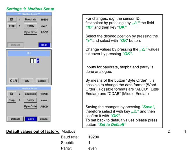
Byte Order: **Remark**: If the sensor is placed at the end of the Modbus system a termination is required. The sensors have an internal switchable termination, therefore the 6 fastening screws from the lid are to be released and set the internal DIP Switch to "On".
